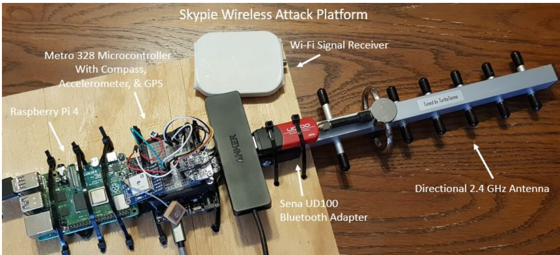
Figure 11: skypie v3 Prototype Hardware Components
