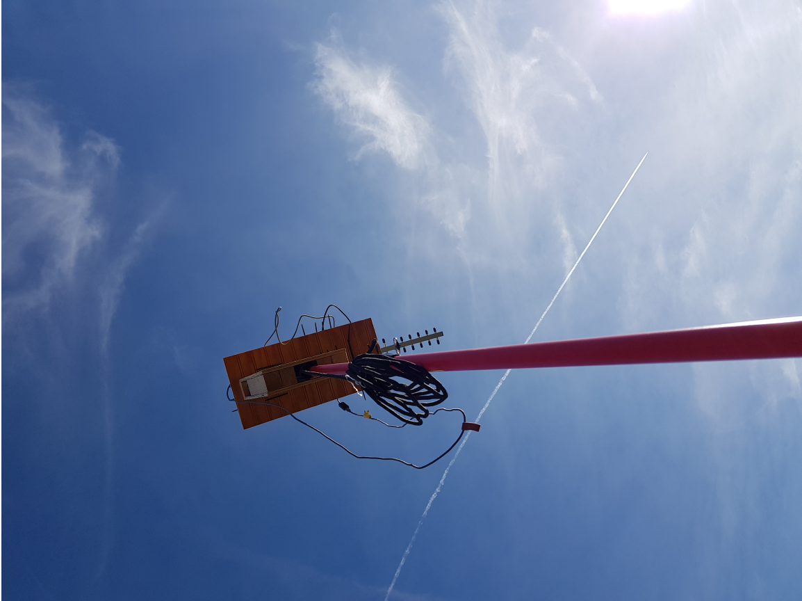
Figure 26: Attack Platform on Pole at 3.05 Meters for Experiment Two.
